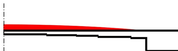
Fig.1 Axisymmetrical model of the back chamber of a miniature microphone
