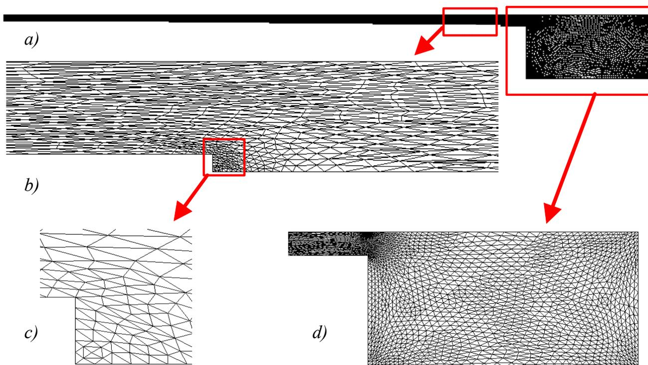
Fig.2 Optimized mesh of the back chamber after 16 mesh adapting iterations a),
