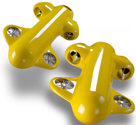
Fig. 1: Prototypes of Serafina MkII AUVs
