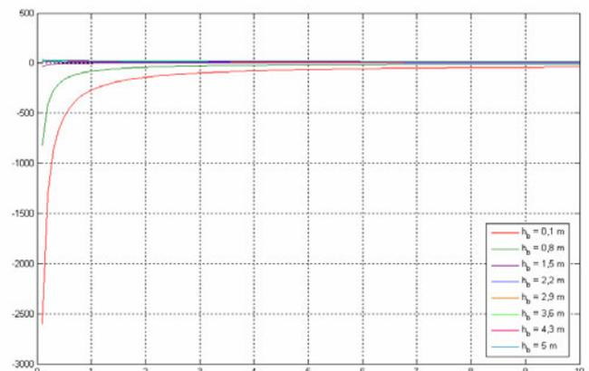
Fig.4 Barrier attenuation variation with constant parameters  $h_s = 0,7$  m;  $R_s = 14$  m;  $R_r = 10$  m;  $C_p = 2$  dB.
