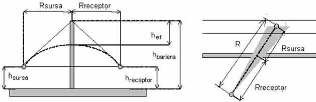
Fig.1 Parameters that determine phonic barrier attenuation.
