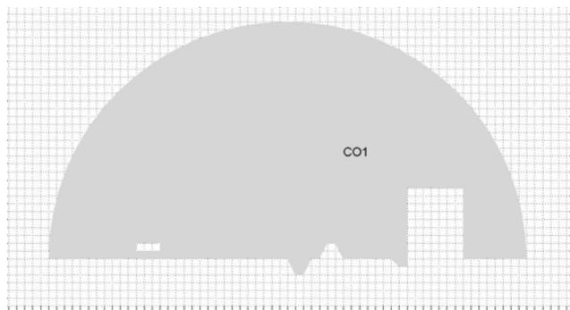
Fig. 10 Model geometry of the road transversal section.
