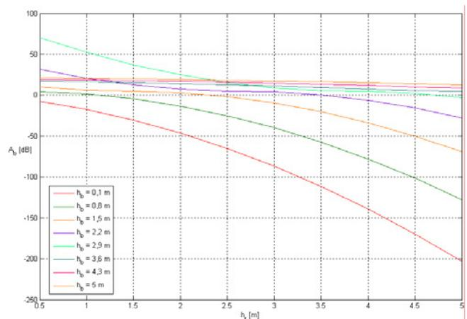
Fig.3 Barrier attenuation variation with constant parameters  $h_s = 0,7$  m;  $R_s = 14$  m;  $R_r = 10$  m;  $C_p = 0$  dB.
