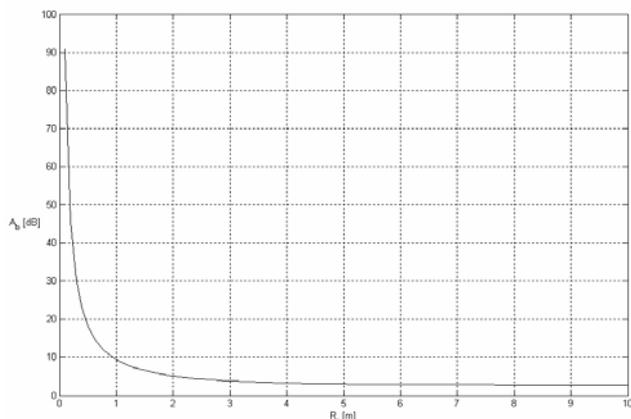
Fig. 8 Barrier attenuation with the source situated at the constant distance  $R_S = 20$  m;  $h_S = 0,5$  m;  $h_T = 1$  m .
