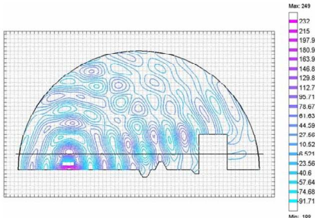
Fig. 12 Sound waves propagation for a source frequency of  $f = 25$  Hz (contour plot).
