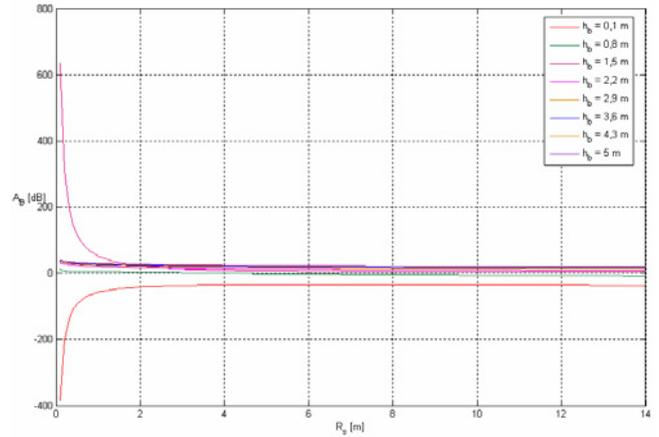
Fig.2 Barrier attenuation variation with constant parameters  $h_s = 0,7$  m;  $h_r = 1,7$  m;  $R_r = 10$  m;  $C_p = 0$  dB.
