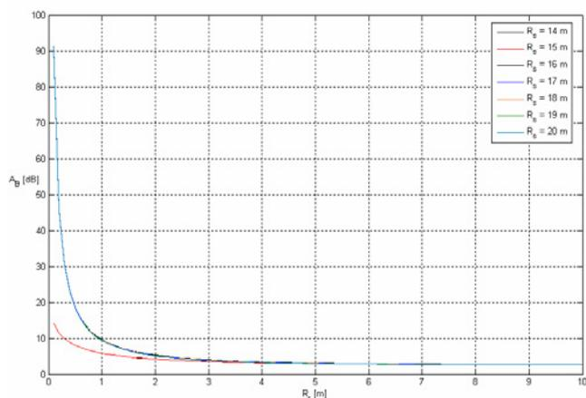
Fig. 9 Barrier attenuation with the source situated at the variable distance  $R_S \in [14;20]$  m;  $h_S = 0,5$  m;  $h_T = 0.7$  m .
