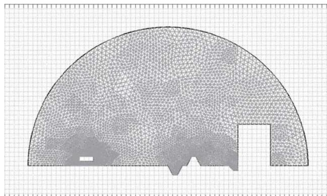
Fig.11 Finite elements mesh.
