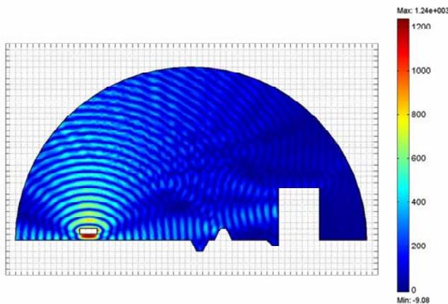
Fig. 13 Sound waves propagation for a source frequency of  $f = 65$  Hz (field intensity display).
