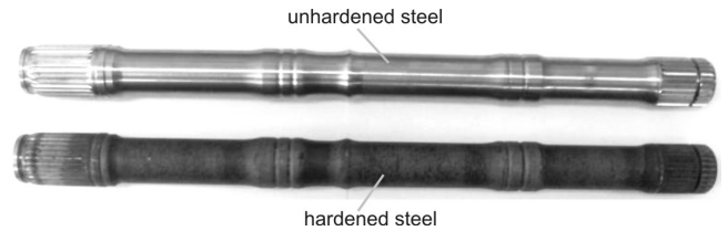
Fig.7. Photograph of a studied cylindrical shaped steel drive shafts.
