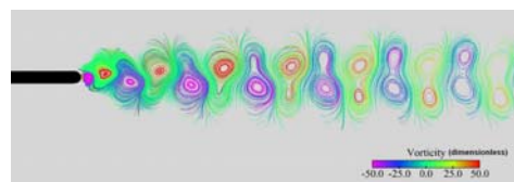
Fig.7: Vortex street St = 0.18 ( Re = 1300 and L_{plate} = 0.1 m)
