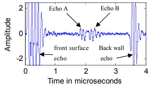
Fig.7 A-scan signal of the part with two echoes.
