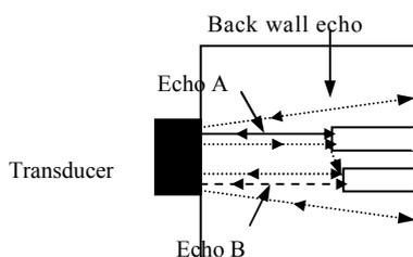
Fig.6 Steel part with two holes leading to the back face.
