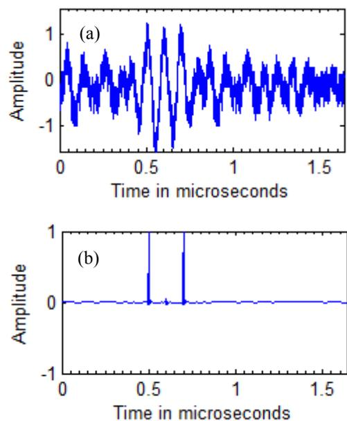
Fig.4 (a) Signal with two echoes drowned in noise separated by  $\Delta\tau=0.2\mu s$  (equivalent to 0.58mm), (b) Results obtained by SSP-NN.
