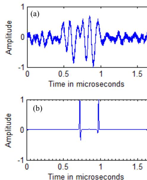
Fig.9 (a) A-scan signal of the part with two distant holes of  $2mm$ , Output of SSP-NN ( $\tau_A=0.71\mu s$ ,  $\tau_B=0.97\mu s$  and  $\Delta\tau=0.26\mu s$ ).
