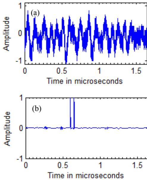
Fig.5 (a) Signal with two echoes drowned in noise separated by  $\Delta\tau=0.05\mu s$  (equivalent to  $0.14mm$ ), (b) Results obtained by SSP-NN.
