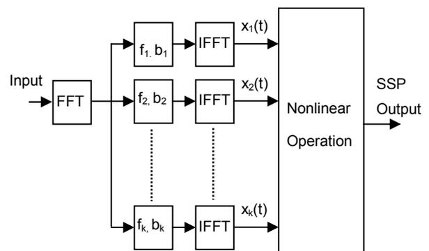
Fig.1 The structure of SSP for generation of k narrowband.
