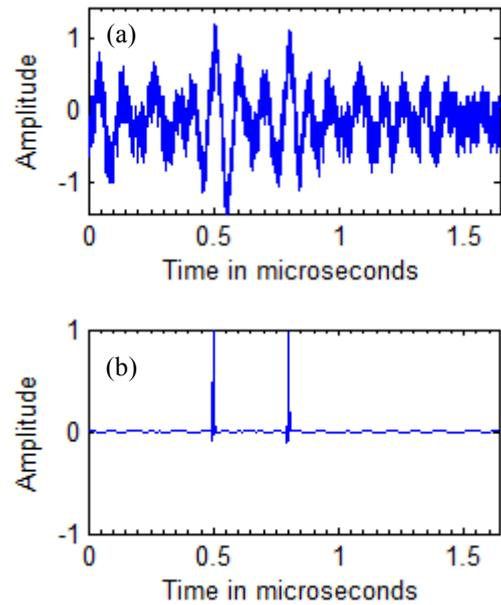
Fig.3 (a) Signal with two echoes drowned in noise separated by  $\Delta\tau=0.3\mu s$  (equivalent to 0.87mm), (b) Results obtained by SSP-NN.
