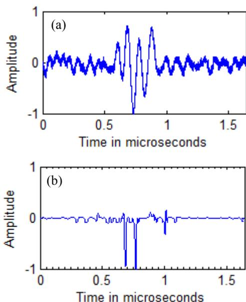
Fig.10 (a) A-scan signal of the part with two distant holes of 1mm, Output of SSP-NN ( $\tau_A=0.7\mu\text{s}$ ,  $\tau_B=0.76\mu\text{s}$  and  $\Delta\tau=0.06\mu\text{s}$ ).
