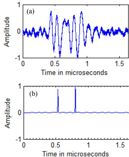
Fig.8 (a) A-scan signal of the part with two distant holes of  $3mm$ , Output of SSP-NN ( $\tau_A=0.53\mu s$ ,  $\tau_B=0.8\mu s$  and  $\Delta\tau=0.27\mu s$ ).
