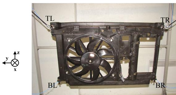
Fig.4. Mounting of the fan system for  $Y_m$  measurement.
