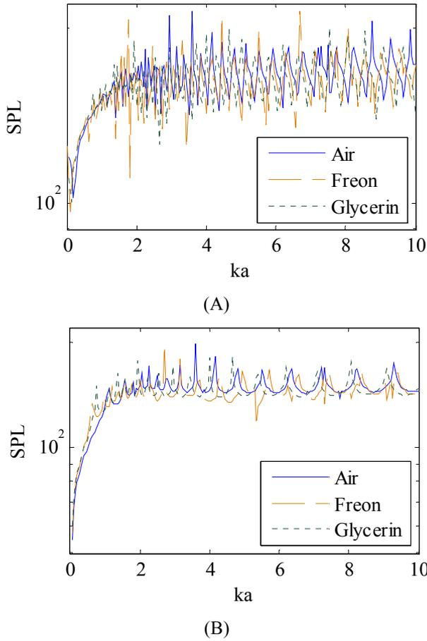
Fig. 3 Sound pressure level on the shell, (A) @  $\theta = 0$ , (B) @  $\theta = \pi/2$  versus frequency
