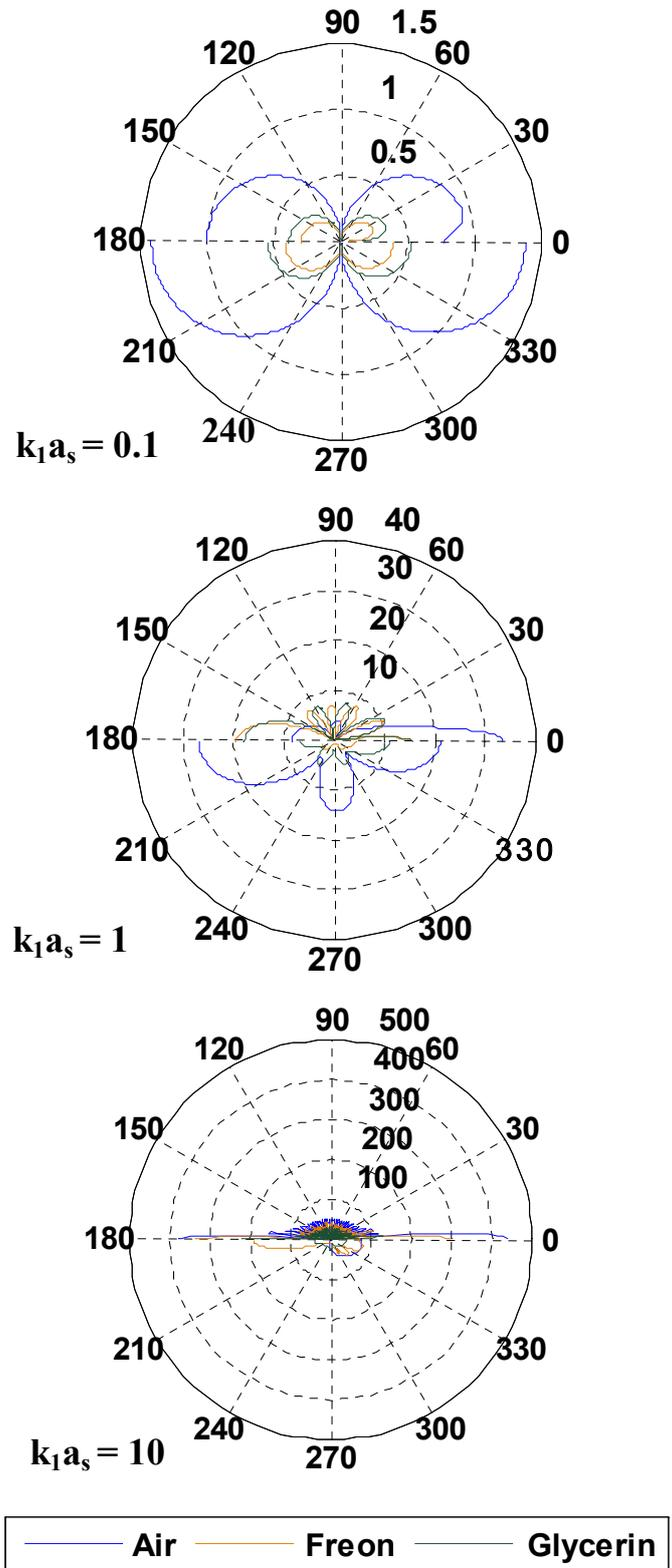
Fig. 2 Near field (@  $r = a_s, 0 < \theta < \pi$ ) and Scaling Far field (@  $r = 10 a_s, \pi < \theta < 2\pi$ ) pressure radiated by the sandwich (Steel-Copper-Steel) spherical shell
