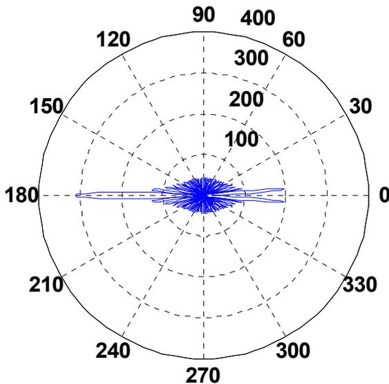
Fig. 4 Pressure on the point excited evacuated single layer spherical shell for  $ka=10$
