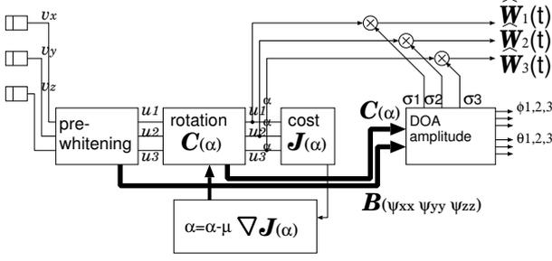
Figure 2: Block diagram of the on-line BSS-DOA processing
