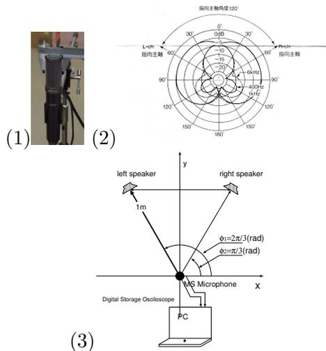
Figure 3: POC-model experimental setup:(1)MS-microphone: SONY ECM-999, (2)the solid curve shows the directional patterns of the L-channel (mid +side ) and the dotted curve shows the R-channel one (mid -side)(dotted curve) microphone from the date-sheet of ECM-999, (3)schematic diagram of the experimental setup.
