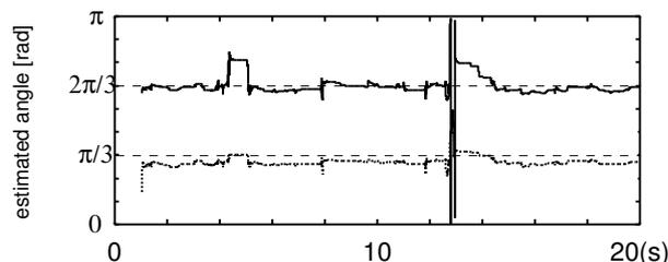
Figure 7: Convergence plots of the estimated directions of the original sound waves: No.1 and No.2.
