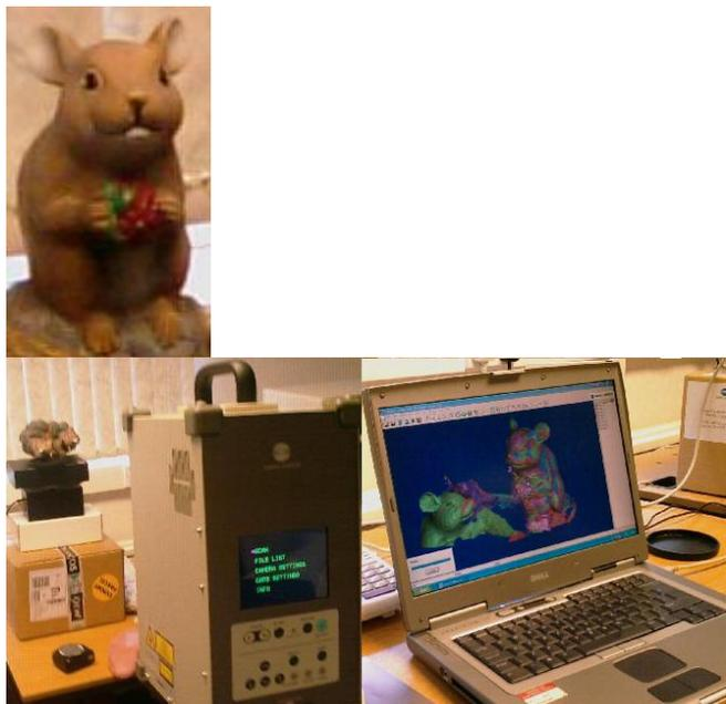
Fig.2. Mouse figurine being scanned and 3D Laser scanner
