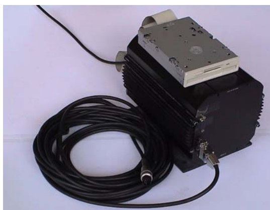
Fig. 3 The signal processing PC-104 cabinet
