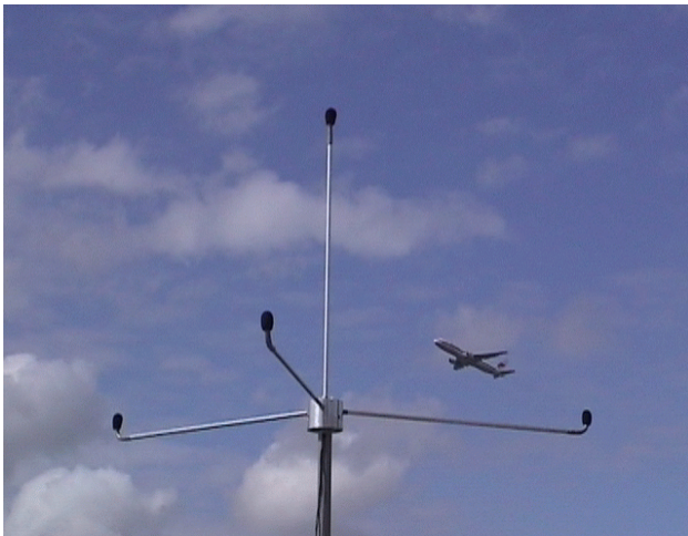
Fig. 1 Four microphones in a spatial configuration for aircraft noise monitoring.
