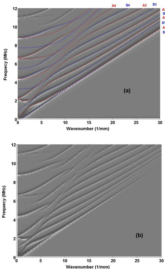
Fig.1 Dispersion spectrum for 1 mm aluminum plate by (a) homogeneous and (b) inhomogeneous (functionally graded) model.
