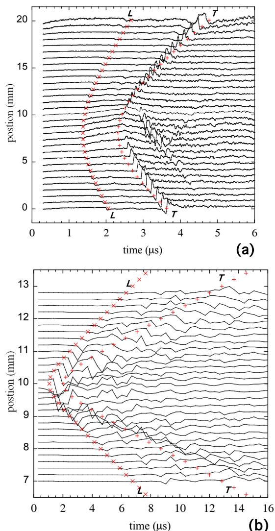
Fig.3 Laser excited transient displacement field : (a) experiment (b) theory for a functionally graded plate.
