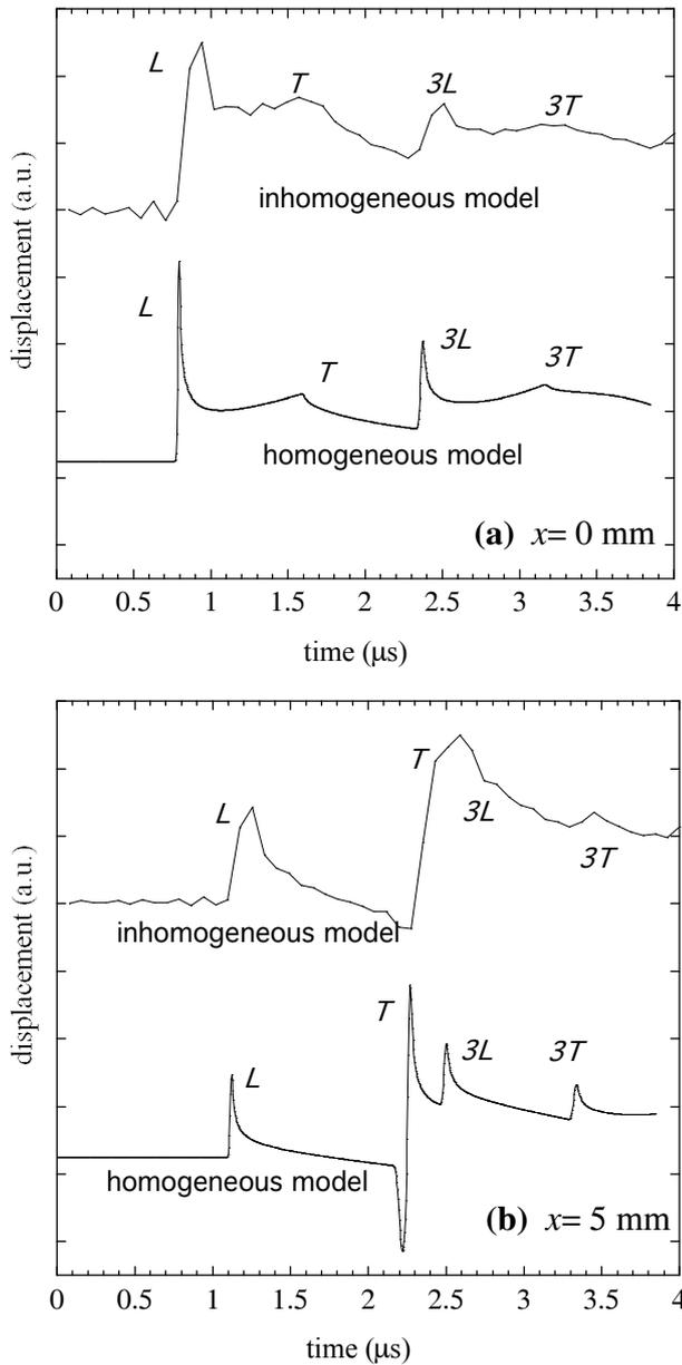
Fig.2 Laser excited transient displacement for a 5 mm aluminum plate calculated at (a) epicenter  $x=0$  and (b) non-epicenter  $x=5$  mm.
