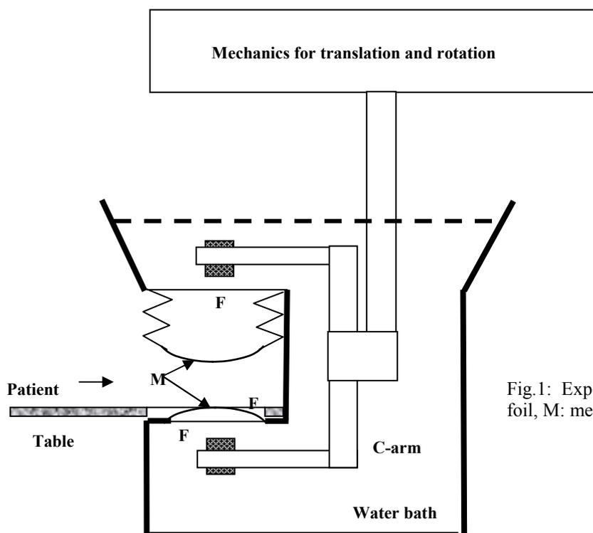
Fig.1: Experimental prototype of the FemUS device (F: foil, M: membrane)
