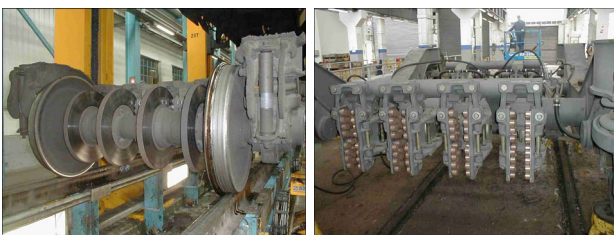
Figure 1: The brake system (discs on the left, linings on the right)
