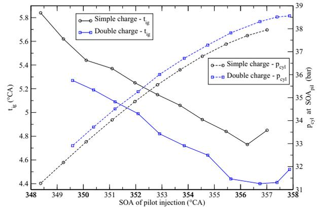
Figure 7: Evolution of the mean ignition delay and the mean cylinder pressure at  $SOA_{pil}$  with the injection timings (for simple and double charge)
