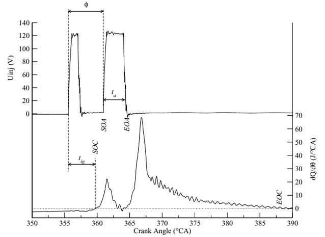
Figure 1: Definition of the start of activation ( $SOA$ ), end of activation ( $EOA$ ), activation duration ( $t_a$ ), time lag between two injections ( $\phi$ ) and ignition delay ( $t_{ig}$ )
