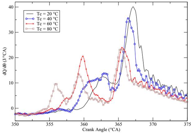
Figure 5: Change in the ROHR shape with the increasing coolant temperature
