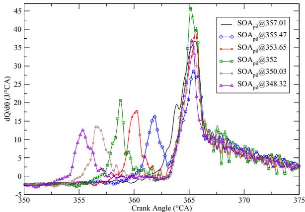
Figure 6: Evolution of the ROHR for several crank angle of  $SOA_{pil}$  (crank angle of  $SOA_{main}$  = constant, simple charge condition)
