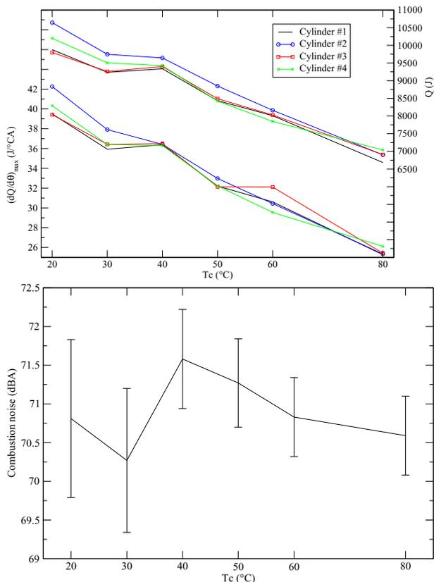
Figure 3: Evolution of the maximum of ROHR, of the integral of ROHR and of the combustion noise with the increase in coolant temperature
