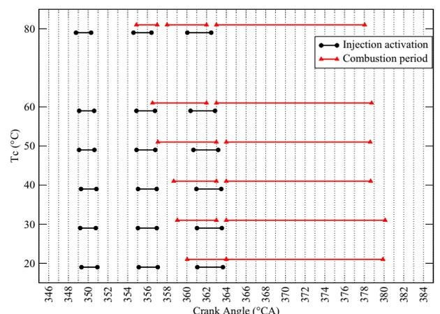
Figure 2: Chart of the injection and combustion timings
