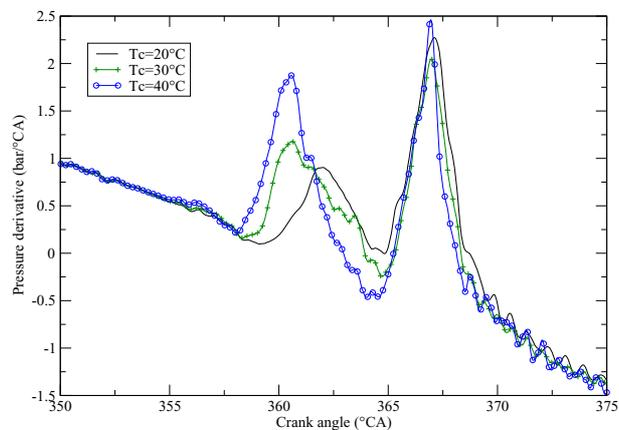
Figure 4: Cylinder pressure derivative analysis at different coolant temperatures -  $T_c = 20, 30$  and  $40^{\circ}\text{C}$
