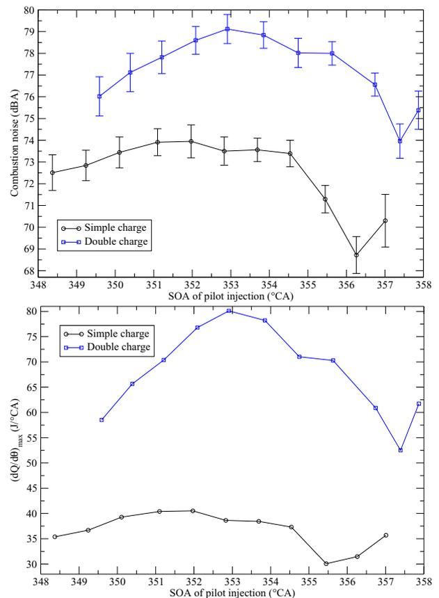
Figure 8: Combustion noise and maximum of ROHR versus  $SOA$  of pilot injection for simple and double charge
