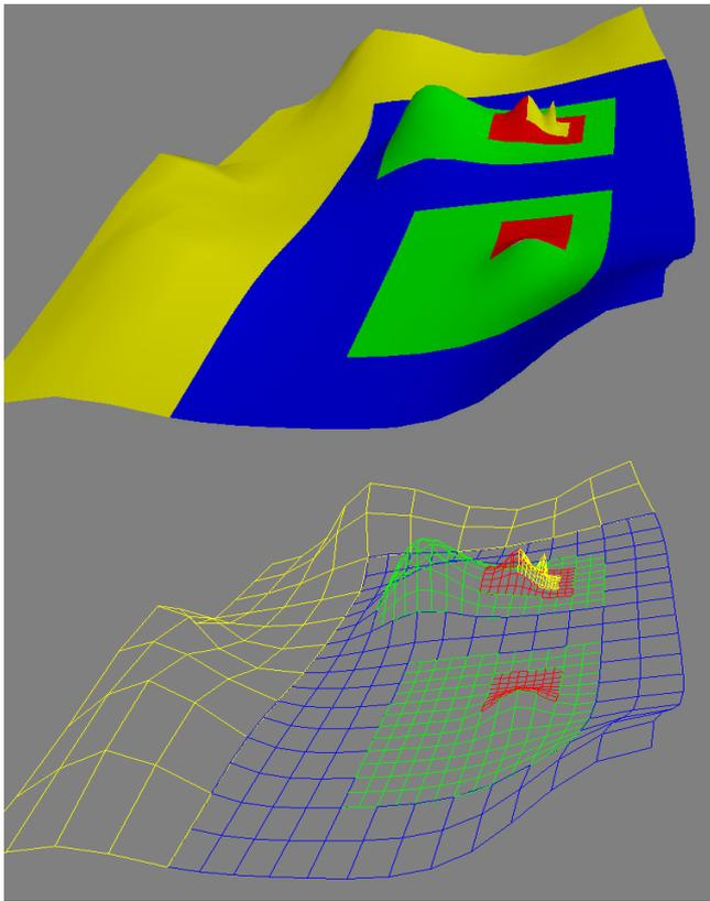
Fig.4. Multiresolution 3D data representation using hierarchical spline function techniques
