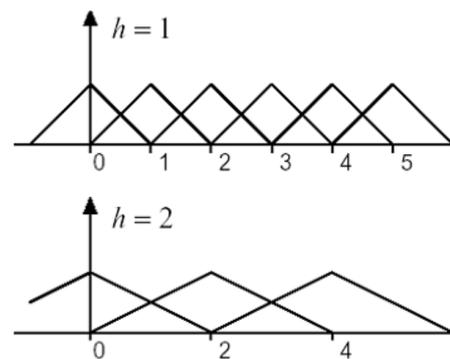
Fig.2a. Knot resolution change in the process of generalization.
