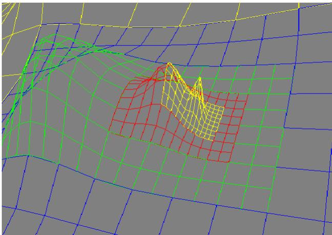
Fig.5. High and low vertical resolution data approximation using hierarchical spline function
