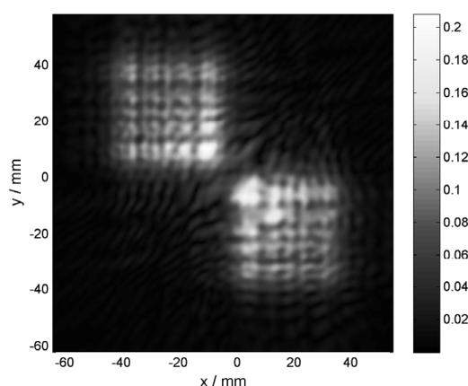
Fig.5 Planar hydrophone scan of PCT quad array.
