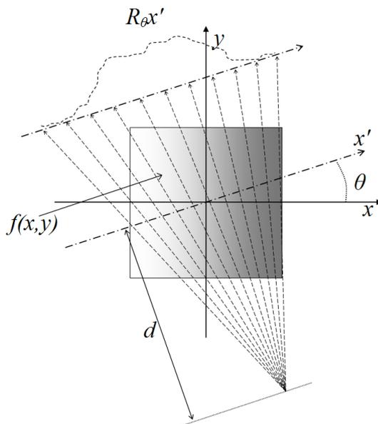
Fig.2 Fan beam scan configuration through some acousto-optic distribution  $f(x,y)$  at an angle  $\theta$ , producing the Radon transform  $R_\theta(x')$ .
