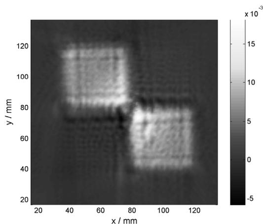
Fig.4 Fan beam acousto-optic scan and reconstruction of PCT quad array.
