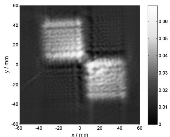
Fig.3 Parallel beam acousto-optic scan and reconstruction of PCT quad array.
