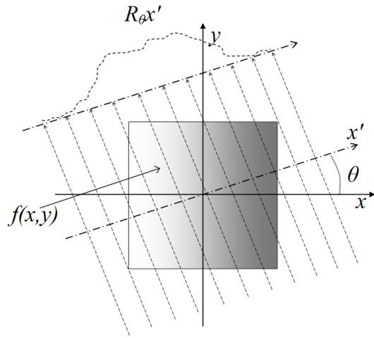
Fig.1 Parallel beam scan configuration through some acousto-optic distribution  $f(x,y)$  at an angle  $\theta$ , producing the Radon transform  $R_\theta(x')$ .
