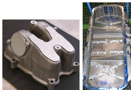
Fig.4 Modified rocker cover and oil sump using sandwich plates and stiffener.
