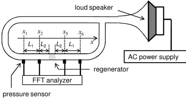
Figure 2: Experimental setup to determine the wave number and thermoacoustic function in the regenerator.
