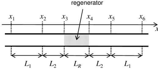
Figure 1: Coordinate system for the experimental evaluation of the wave number in the stacked-screen regenerator.
