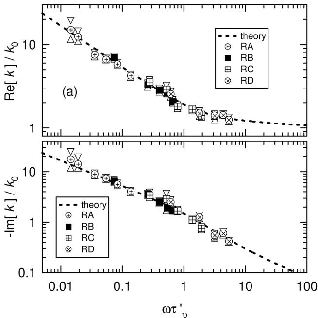
Figure 4: The experimental results of the wave number  $k_{exp}$  in the stacked screen regenerators. The wave number  $k_{exp}$  is shown as a function of the modified  $\omega\tau'_\nu (= \omega\tau_\nu/f)$
