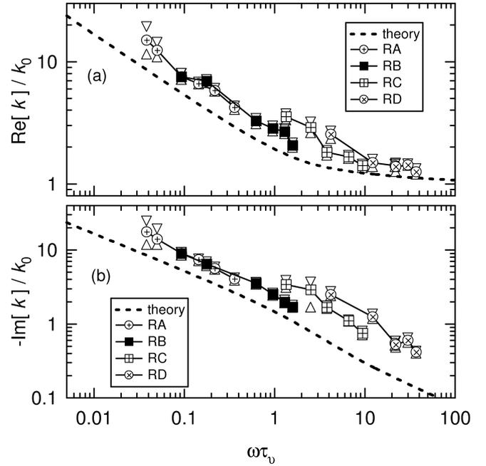
Figure 3: The experimental results of the wave number  $k_{exp}$  in the stacked screen regenerators. The wave number  $k_{exp}$  is shown as a function of  $\omega\tau_\nu$
