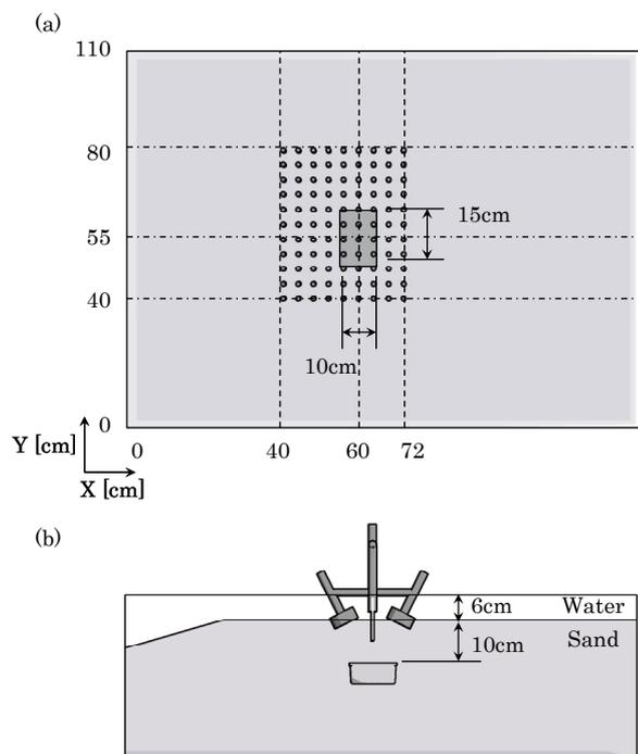
Fig. 8. Outline of the experiment for three dimensional image: (a) Top view. Small circles in this figure show measurement points, (b) Side view. Focal length is adjusted to buried depth of the target.
