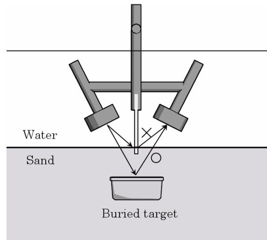
Fig. 1. Our exploring method with ultrasounds emitted from the water. The acoustic shielding board placed in the middle of the transducers block direct wave and reflected wave from the ground surface.
