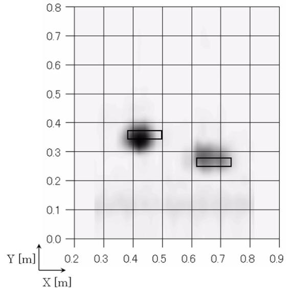
Fig. 7. Under ground image at the depth of 3 cm in water tank.
