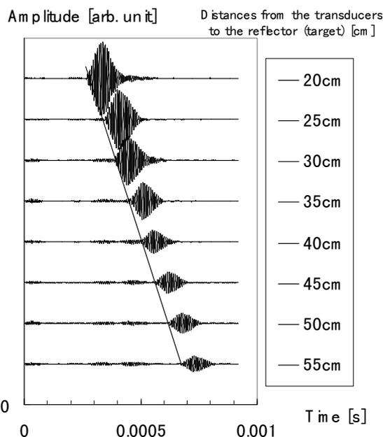
Fig. 4. Reflected waves at each distance. Slope of an oblique line shows the propagating velocity of about 1500m/s.
