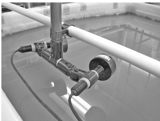
Fig. 2. The picture of transducers fixed with the pipes. The focal length is variable.
