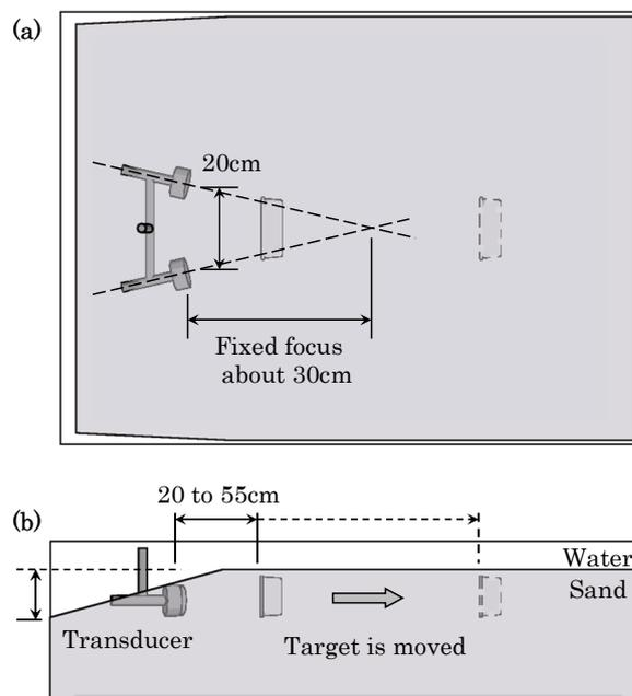
Fig. 3. Outline of the experiment for measurement of propagation property: (a) Top view, (b) Side view.
