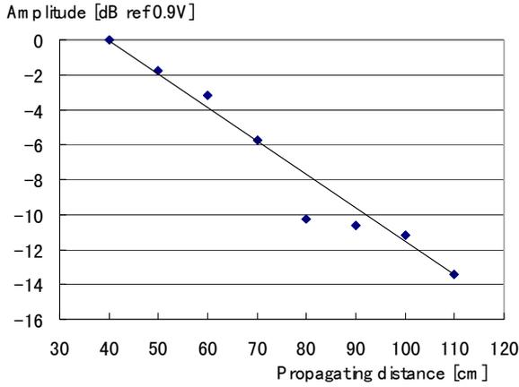
Fig. 5. The attenuation of ultrasound. Slope of an oblique line shows the attenuation of about -19 dB/m.
