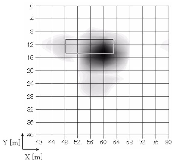
Fig. 10. Cross section where x is 56 cm. A rectangle line shows size and buried point of the target.
