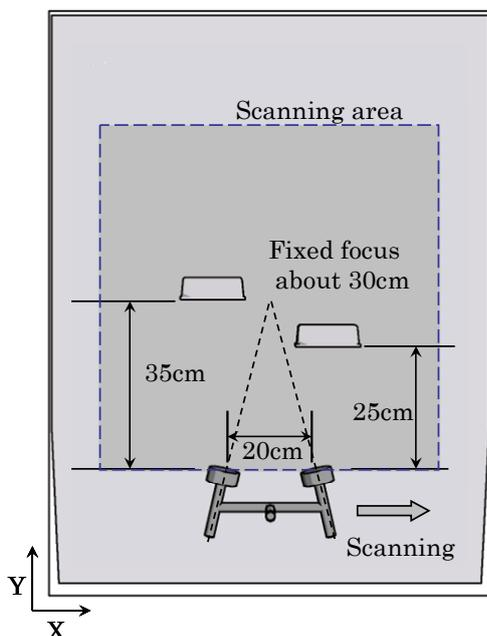
Fig. 6. Top view of the experiment for the B mode imaging. Square written in broken line shows scanning area.
