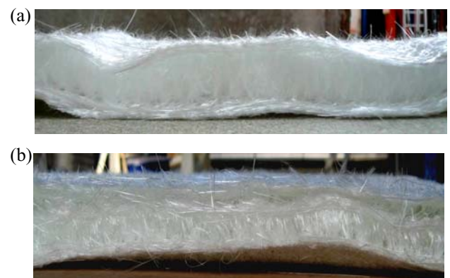
Fig.5 3D NAPCO structures without PCM; (a) two mat and (b) three mat structures.
