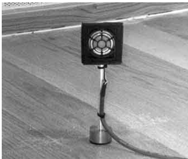
Fig. 7 Miniature loudspeaker used in the physical scale model
