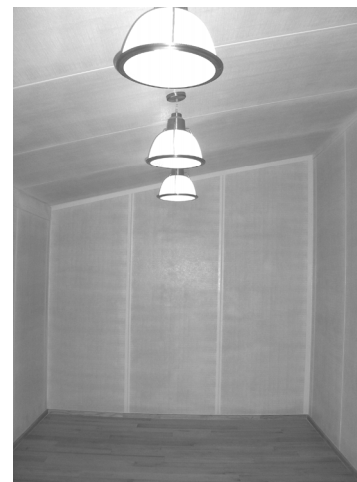
Fig. 2 Interior of the hemi-anechoic chamber
