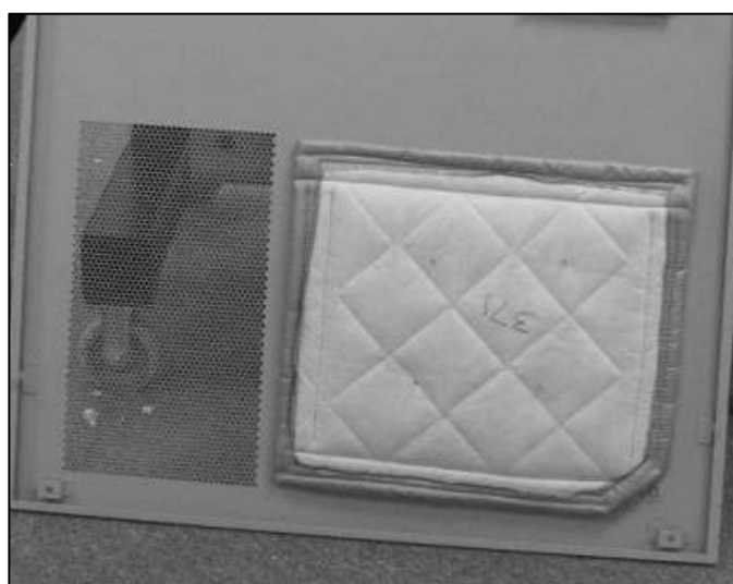
Figure 6. DuPont™ LoWave™ treatment mounted on housing panels.
