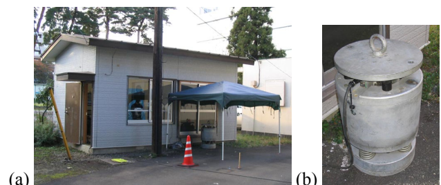
Fig.1 (a) test house and (b) exciter used in experiment.
