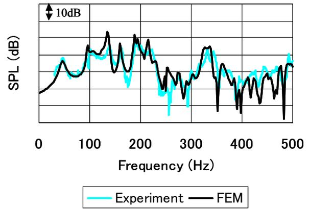
Fig.17 Validation of floor FE model (Absorptive type)
