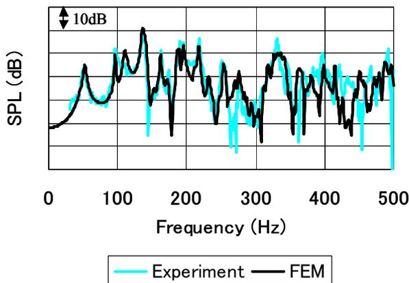
Fig.15 Validation of floor FE model (without carpet)
