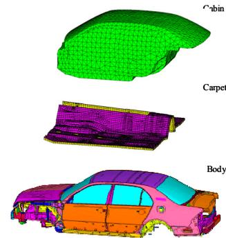
Fig.12 FE model for validation
