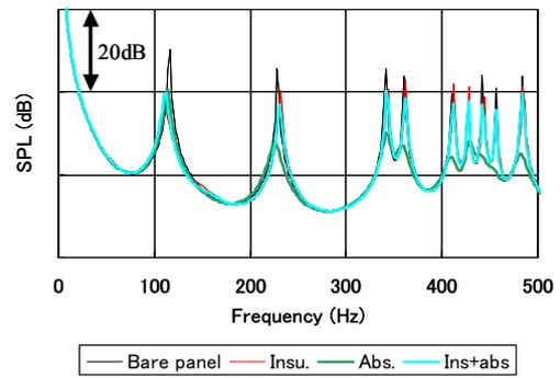
Fig. 10 Sound absorption of porous trims
