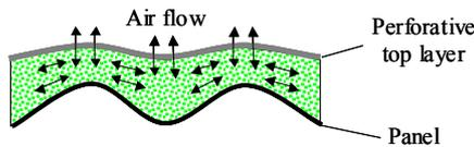
Fig. 8 Vibration mode of absorptive trim
