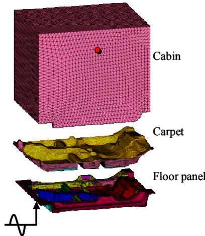
Fig.14 Floor panel with carpet FE model
