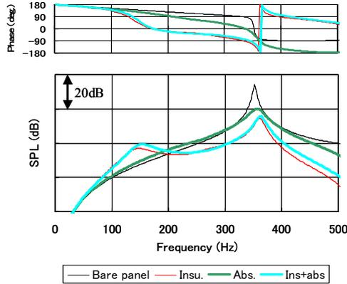
Fig. 7 Sound radiation of porous trims
