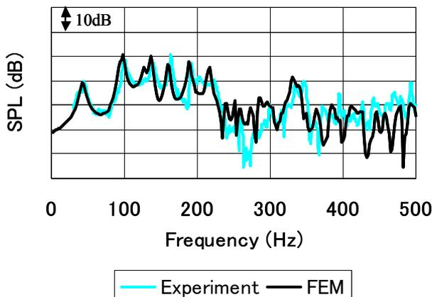
Fig.16 Validation of floor FE model (Insulative type)
