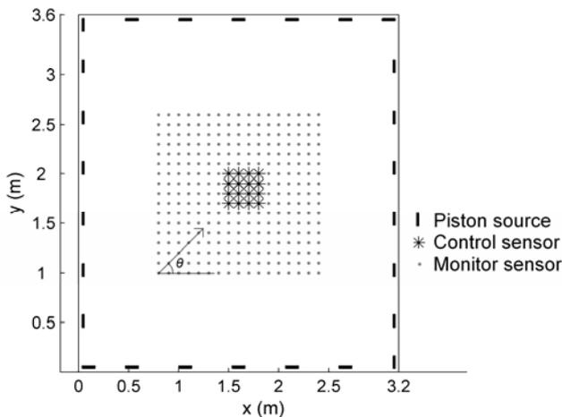
Fig.1 Geometry of the room and arrangement of the sound reproduction system.
