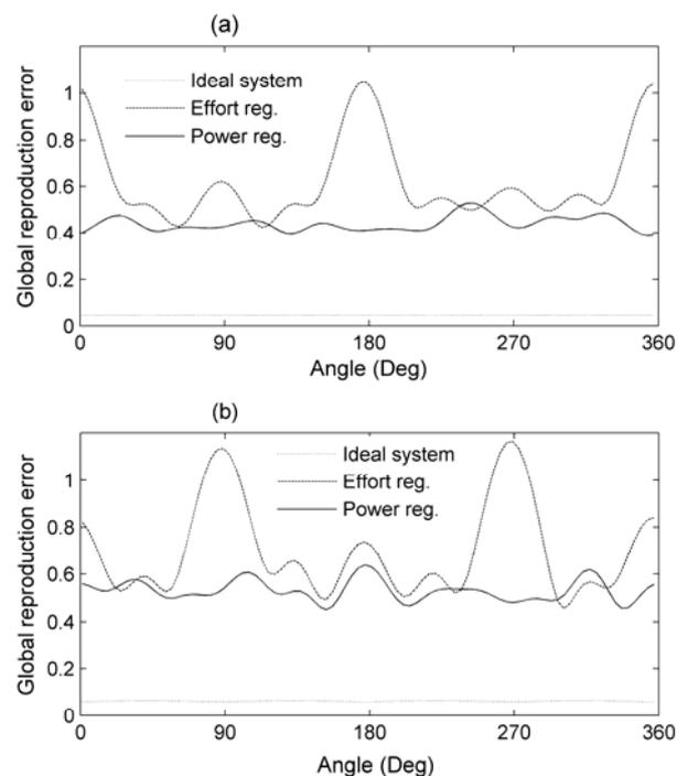
Fig. 2 Global reproduction performance as a function of the angle of propagation of the plane wave at **a.** 330 Hz and **b.** 400 Hz.
