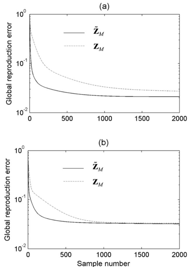
Fig. 5 Global reproduction error as a function of the iteration number of the adaptive algorithm for the generation of a plane wave traveling **a.** at  $90^\circ$  at 160 Hz and **b.** at  $0^\circ$  at 220 Hz.
