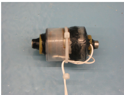
Fig. 13 Constructed back-to-back transducer with plastic baffle.
