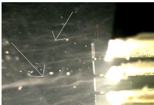
Figure 11: Dense bubble structure (left arrow) ahead of the membrane module, lighter (right arrow) streamers flow around the membrane module. P_e=1.5 \text{ W/cm}^2 , 130 kHz. Measurements of Fig. 10 were carried out between the two lower membrane sheets.
