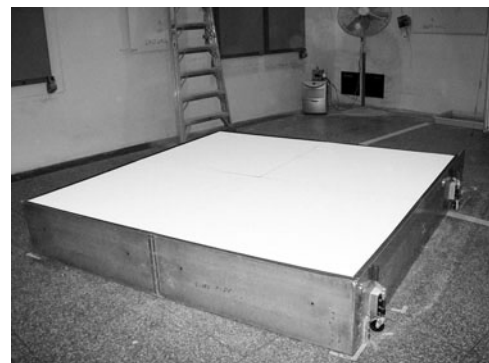
Figure 1b: Sample mounted in E-400 test fixture, 64 ft 2
