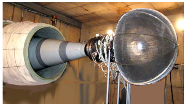
Fig. 4. Test rig and turbulence control screen (TCS).
