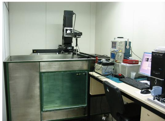
Fig. 1. General view of the ultrasonic pressure mapping system. On the background, the water bath can be seen.
