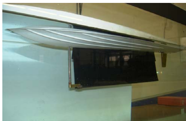
Fig.3 Under-water view of the hull and the assembled propulsive plate.
