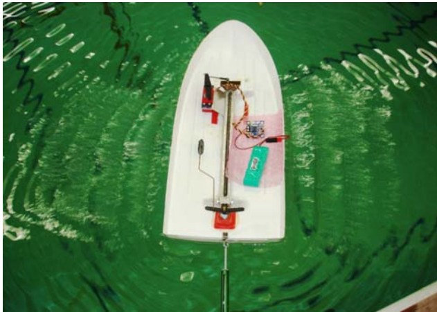
Fig.5 Static thrust test in progress
