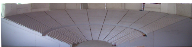
Fig.1 The scale model of Siracusa theatre in the bare configuration (cavea only).
