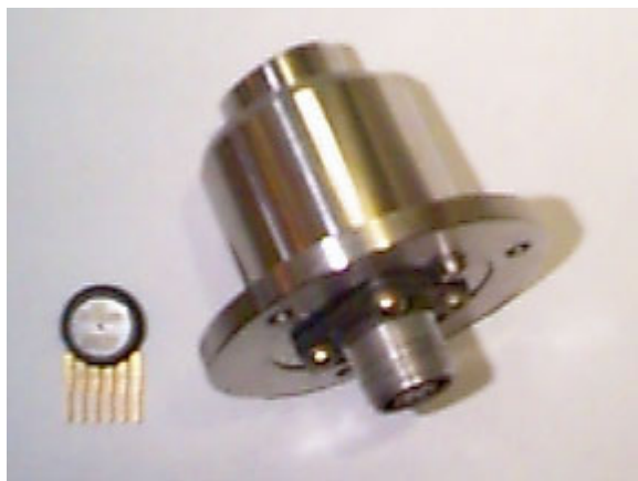
Fig.1 The pressure sensor Motorola type MPX 50-10 and the reference transducer.
