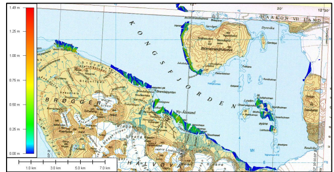
Fig.5. Preliminary map of algae distribution and height variability in Kongsfjord, based on BioSonics DTX measurements. The colourbar intensity is related to the height [m] of algae, which reaches 1.5m in some places.
