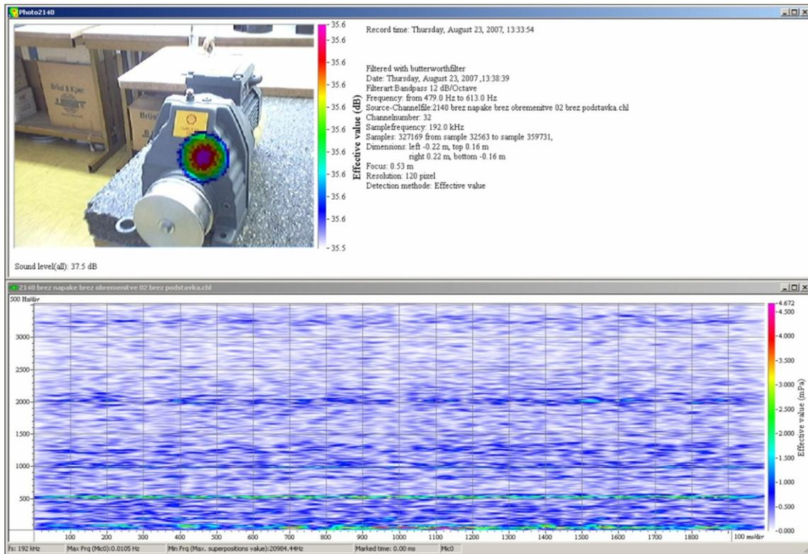
Fig. 5. Acoustic image with spectrogram of a faultless gear
