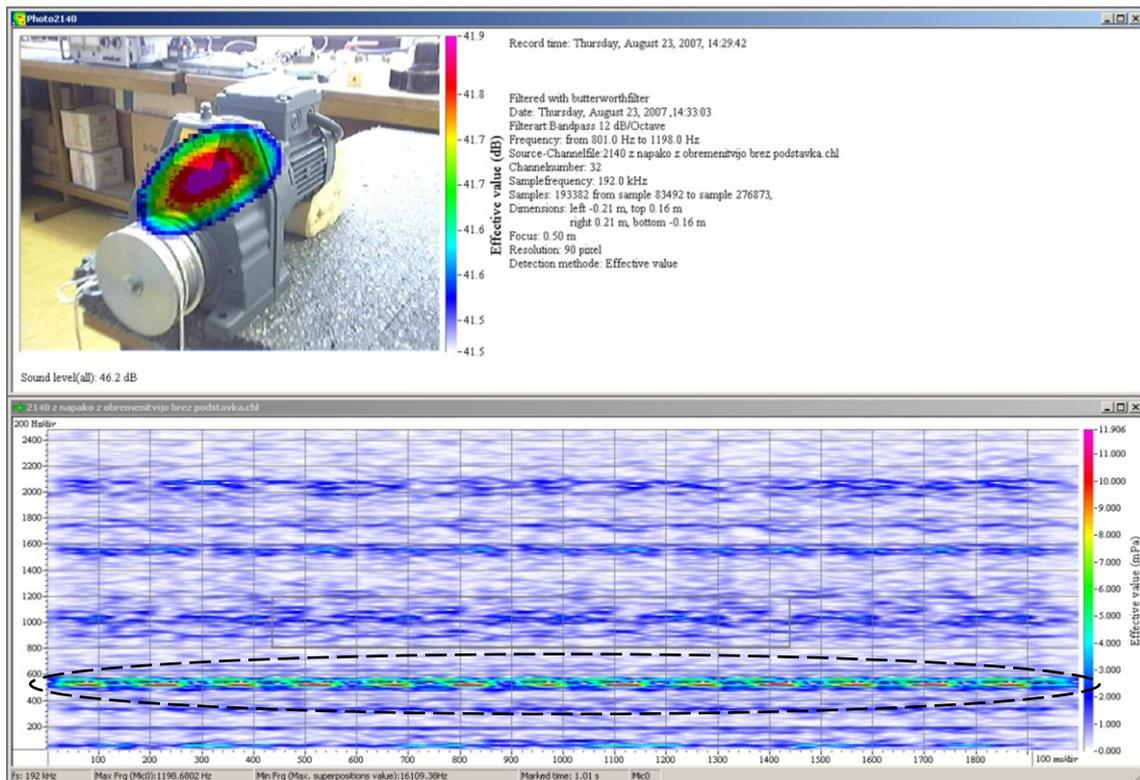
Fig. 6. Acoustic image with spectrogram of a gear unit with a notch in the tooth root
