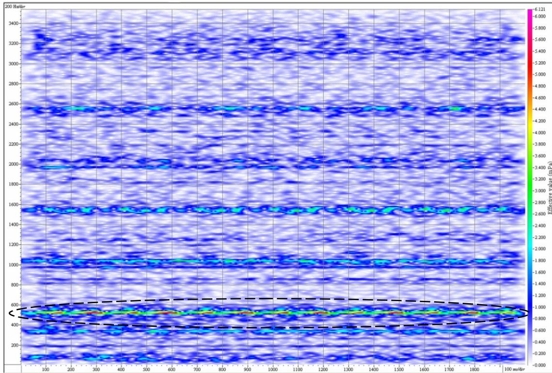
Fig. 7. Spectrogram of a gear unit with a notch in the tooth root, position 4
