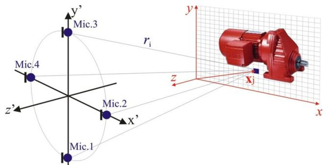
Fig. 1. Length of the path of an elementary source to individual microphones located on an acoustic camera
