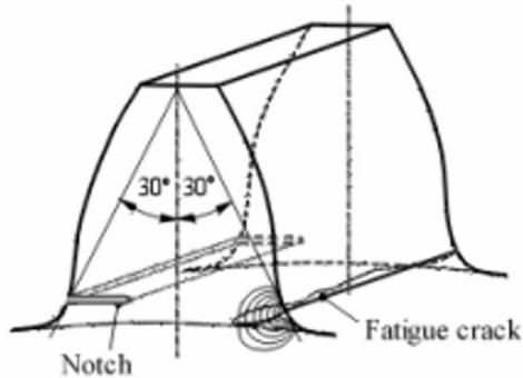
Fig. 3. Differences between a notch and a fatigue crack in a tooth root
