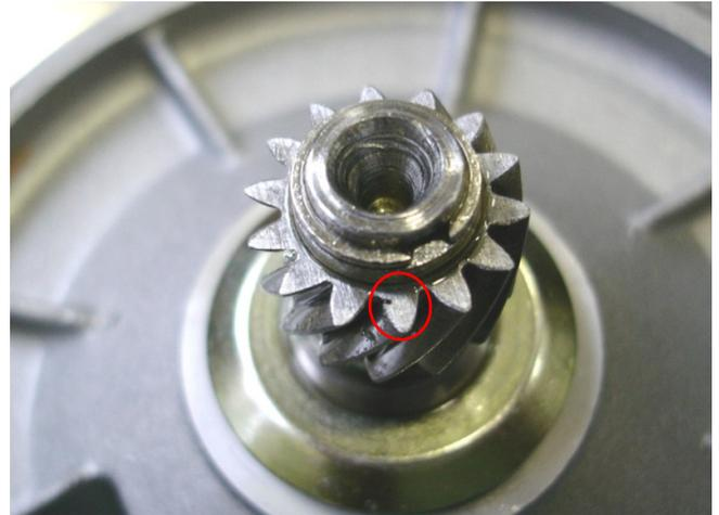
Fig. 4. Pinion with a notch in the tooth root
