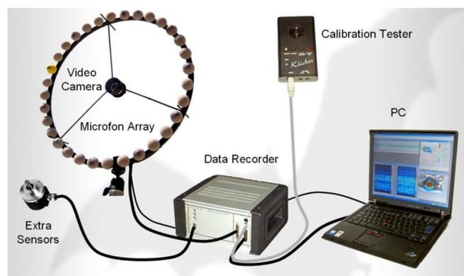
Fig. 2. An acoustic camera system GFaI for visualisation of acoustic sources
