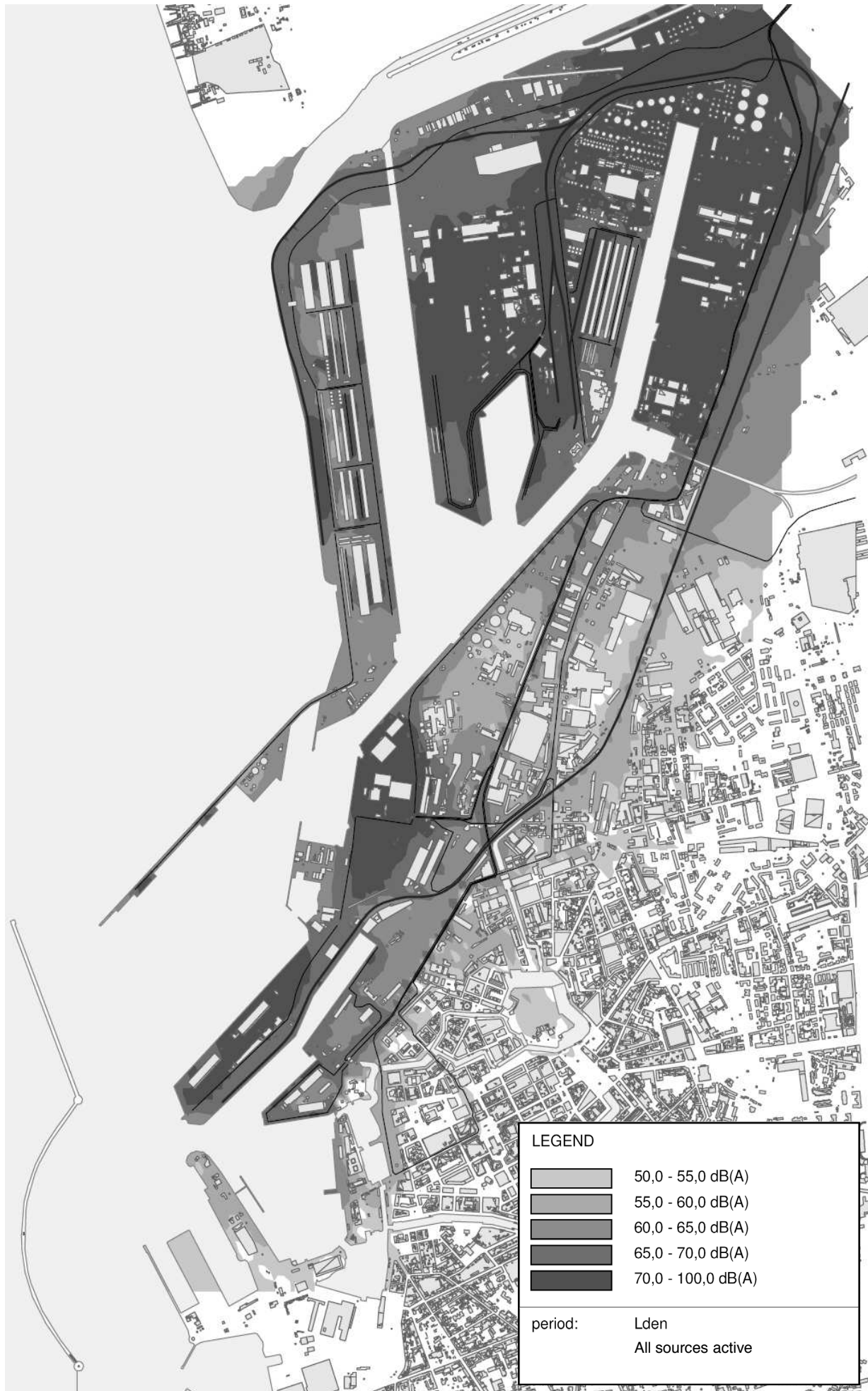
Fig.4. Port of Livorno noise mapping: overall L_{den} levels at 4 metres height.
