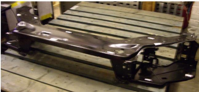
Figure 6: Grill Over-hanging Reinforcement (GOR)
