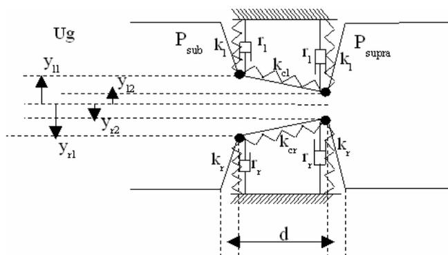
Fig.1 Two mass mode of vocal folds or trombonist lip's.  $U_g$  is the volume flow rate.  $P_{sub}$  is the upstream pressure.  $P_{supra}$  is the downstream pressure.  $L_g$  the constriction width,  $d$  constriction length.  $y_{11}$ ,  $y_{12}$ ,  $y_{21}$ ,  $y_{22}$  are the mass positions compared to the central axis.  $k_1$  and  $k_r$  are the spring
