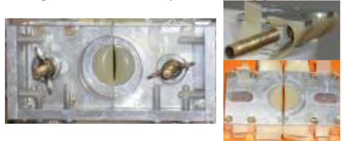
Fig.3 Picture of the oscillating replica. Metallic pieces are covered by latex of  $0.3\text{mm}$  thickness and filled with water under controlled pressure.
