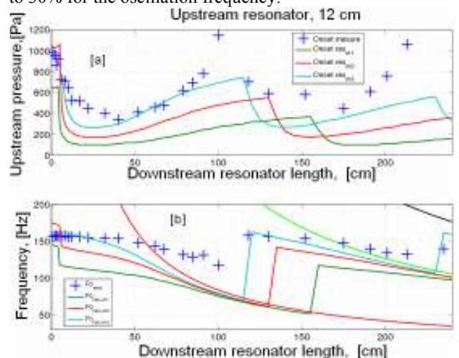
Fig.5 Comparison between theoretical prediction and experimental data, for an upstream resonator of 12cm length, and a downstream resonator of varying length (0 to
