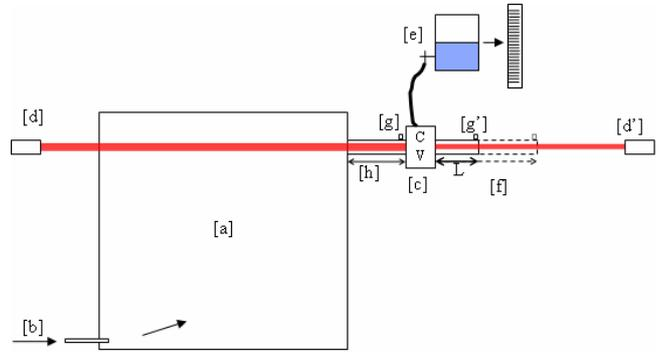
Fig.2 Experimental set-up. [a] Pressure reservoir (lungs). [b] Air supply. [c] Vocal fold/lips replica. [d][d'] Laser diode and photo sensor. [e] Water pressure reservoir. [f] Downstream resonator of variable length. [g][g'] Pressure sensors. [h] Upstream resonator of fixed length.
