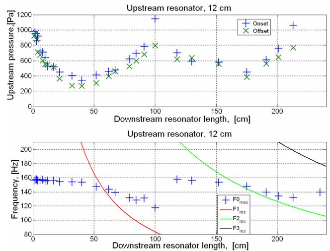
Fig.4 Experimental measurement of the downstream resonator influence. [a] Upstream pressure thresholds. Upstream pressure is increased until oscillations appear (+ Onset pressure). Then pressure is decreased until oscillations cease (x Offset pressure). [b] Fundamental frequency of oscillations. The continuous lines represent the theoretical resonance of the downstream resonator.
