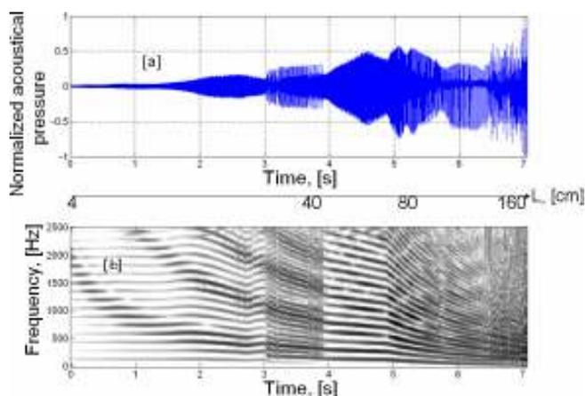
Fig.6 Dynamical simulation. The length of the downstream resonator is time-varying from 4 to 160cm. [a] Normalized acoustical pressure. [b] Spectrogram of the normalized acoustical pressure.
