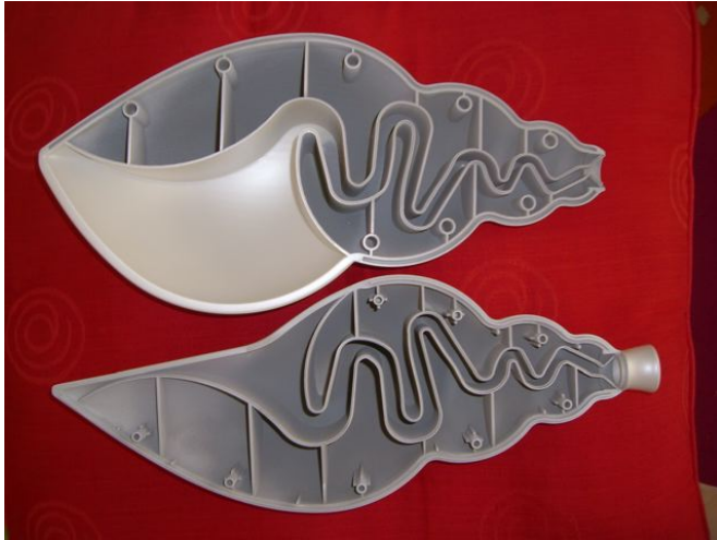
Fig.11: picture of the two parts of the artificial conch, made in rapid prototyping. The inner shape of the bore is visible in the two half-parts.
