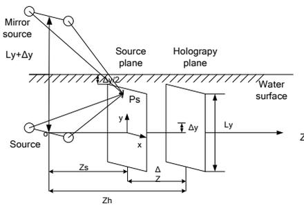
Fig.4 The plane to plane holographic transforms model of two sound sources
