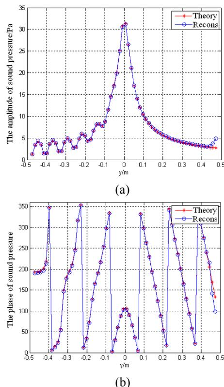
Fig. 2 The comparison between the reconstructed sound pressure field from equation (7) and that from point source formula on source plane.
