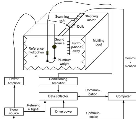
Fig.6 The disposal diagram of experimental system.
