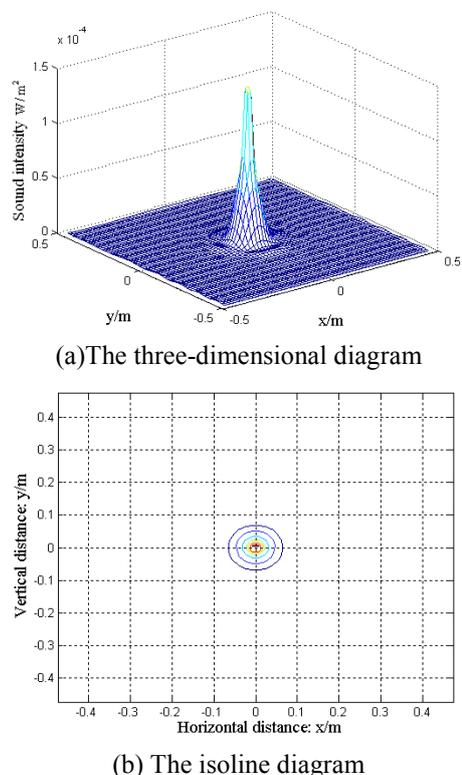
Fig.3 The three dimensional diagram and isoline diagram of reconstructed sound intensity distribution in source plane
