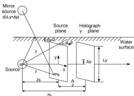
Fig.1 The plane to plane holographic transforms model for single source
