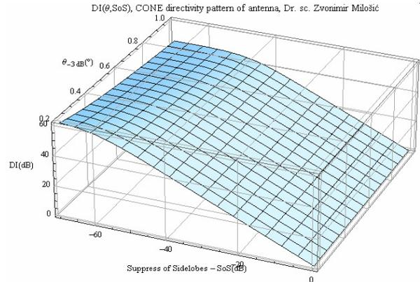
**Fig. 3.5** Graphical presentation  $DI(\theta, SoS)$  of measured conical directivity pattern of ring antenna.
