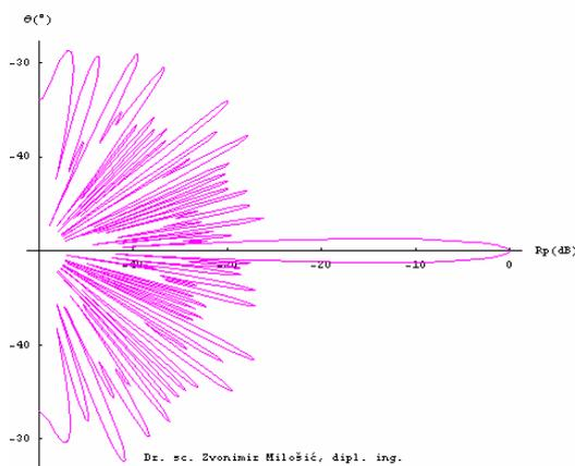
Fig. 2.2 Measured or simulated directivity cone patterns of sonar antenna in one plane, if we have angle  $\theta_{-3dB}=1^\circ$  with suppress of side lobes  $SoS=-25$  dB we have  $DI_{SoS}=+25$  dB.
