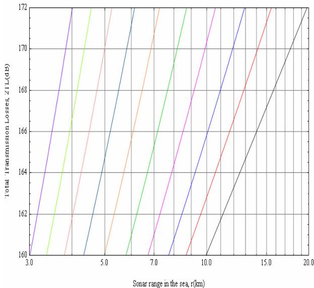
**Fig. 3.7** The graphical presentation of the impact of change of total transmission losses  $2TL(\alpha, r)$  on the change of sonar range  $r$  to Thorp in literature [13].
