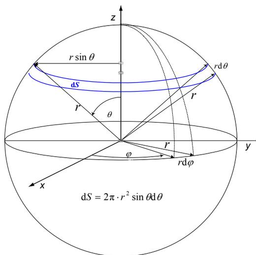
Fig. 3.1 Model of the coordinate system for de-embedding of any parameters the new modern sonar antennas with the cone directivity pattern characteristics.
