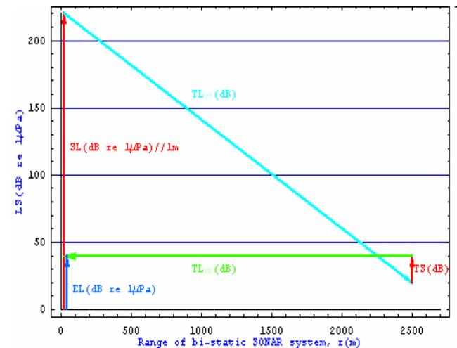
**Fig. 1.1** The symbolical presentation of the importance levels with sonar systems in the sea, from the transmit antenna to the target and back, from the target to the antenna in receive.
