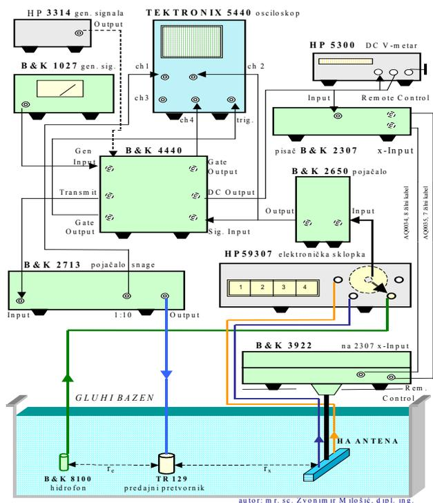
Fig. 2.1 Block scheme for measurement of directivity pattern characteristic  $R_f(\theta_{-3dB}, SoS)$  of hydroacoustical antenna in the receive.
