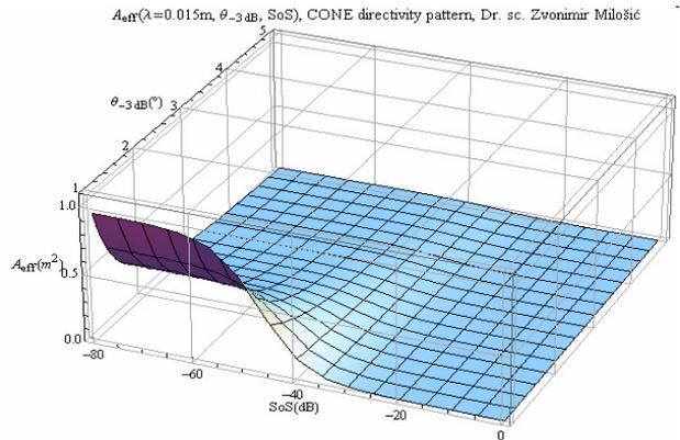
**Fig. 3.6** Graphical 3D presentation of effective aperture area of conical directivity pattern of concentric ring antenna as function  $A_{eff}(D_f, \lambda)$ , to equation (3.14) and to literature [1, 2, 3, 10, 11, 12]
