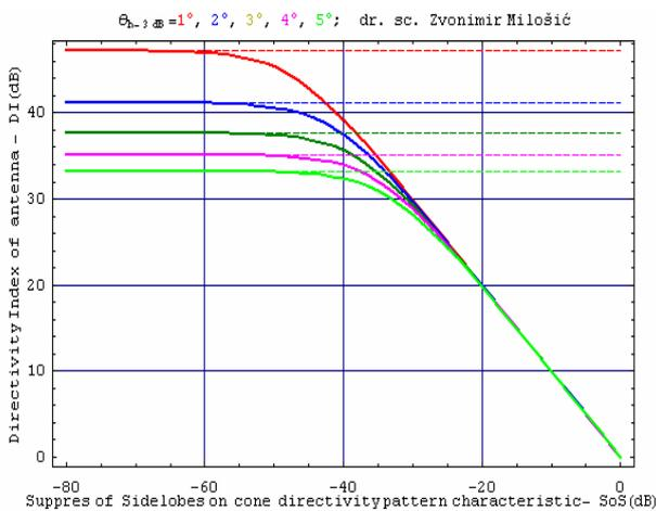
**Fig. 3.4** Graphical presentation  $DI(\theta, SoS)$  of conical directivity pattern of concentric ring antenna as function of sensitivity angles  $\theta_{-3dB}$  and level of suppression of side lobes  $SoS$ .
