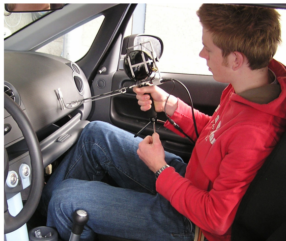
Fig. 9: The novel technique to measure the reflection coefficient of acoustic damping materials can be used in situ.
