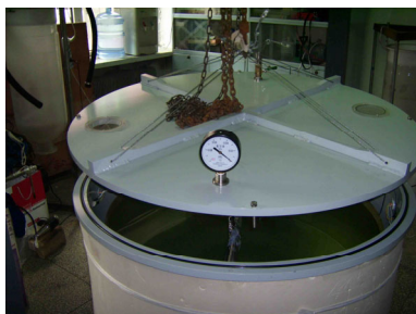
Fig. 2 The design of vibration isolation and degassing
