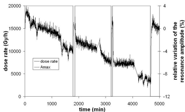
Fig. 5 Effect of gamma radiation for the resonance amplitude  $A_{\max}$  of a 0,6mm thin PZ27 piezoelectric cell in free mode
