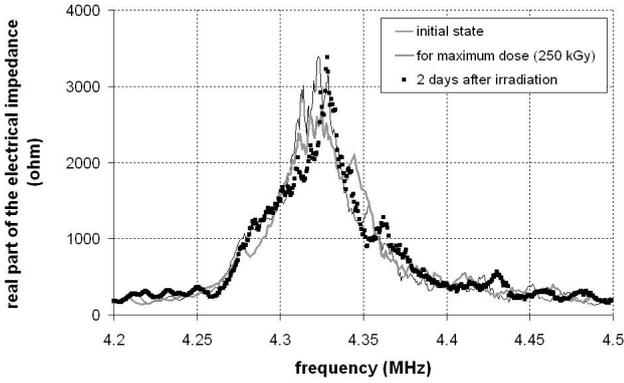
Fig. 8 Effect of gamma radiation on the electrical impedance of a PZT43 cell in free mode
