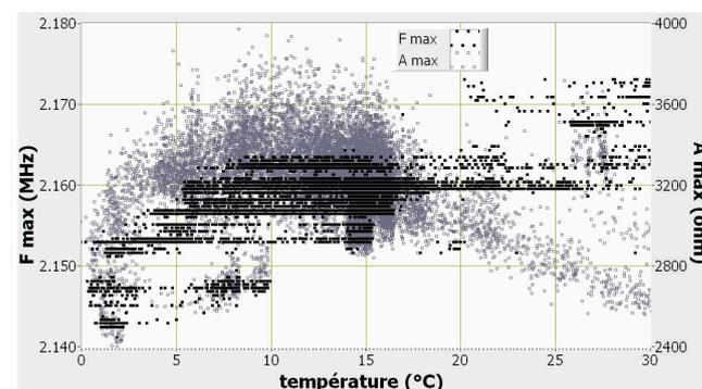
Fig. 15 Correlation of the electrical resonance parameters to temperature variation during irradiation campaign for the 1mm thick PZT27 piezoelectric cell in free mode
