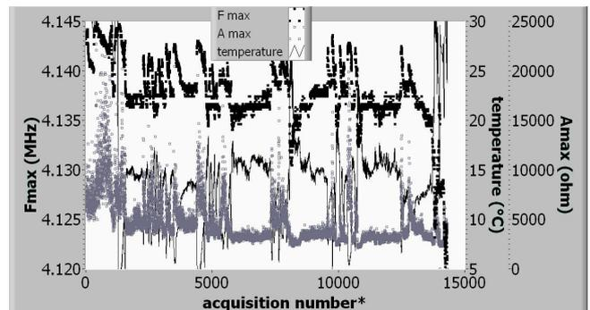
Fig. 11 Neutron irradiation test for a 0,6mm thin PZT46 piezoelectric cell in free mode
