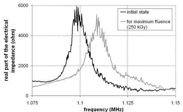
Fig. 2 Effect of gamma radiation on the electrical impedance of a 2mm thick PZ27 cell in free mode
