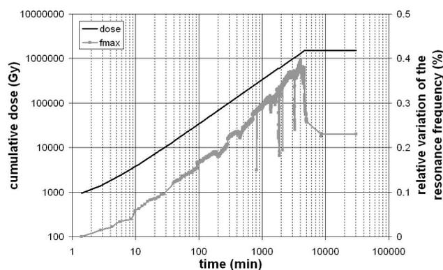
Fig. 4 Effect of gamma radiation for the resonance frequency  $F_{\max}$  of a 0,6mm thin PZ27 piezoelectric cell in free mode
