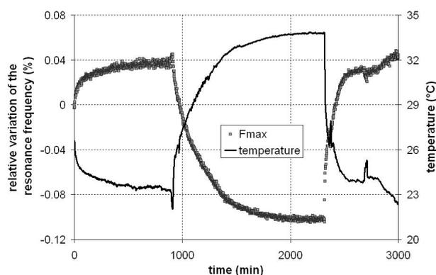
Fig. 14 Temperature dependence of the resonance frequency  $F_{\max}$  for the 0,5mm thin PZT46 piezoelectric cell
