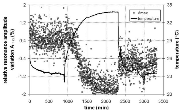
Fig. 6 Temperature dependence of the resonance amplitude  $A_{\max}$  for the 0,6mm thin PZ27 piezoelectric cell
