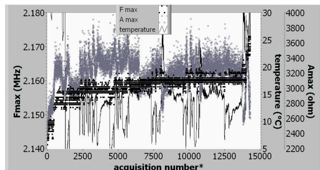
Fig. 12 Neutron irradiation test for 1mm thick PZT27 cell in free mode
