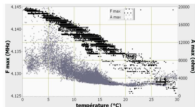
Fig. 13 Correlation of the electrical resonance parameters to temperature variation during irradiation campaign for the 0.5mm thin PZT46 piezoelectric cell in free mode
