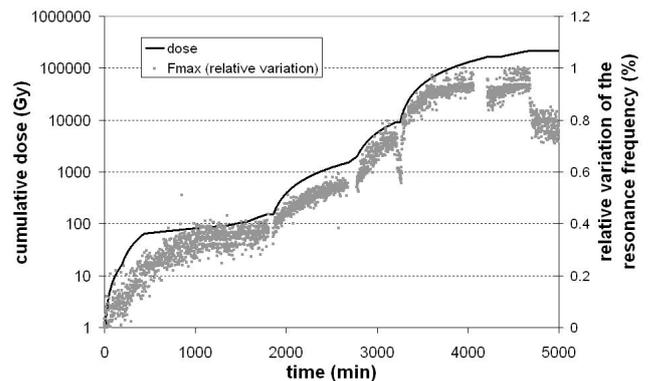
Fig. 1 Effect of gamma radiation for the resonance frequency of a 2mm thick PZ27 cell
