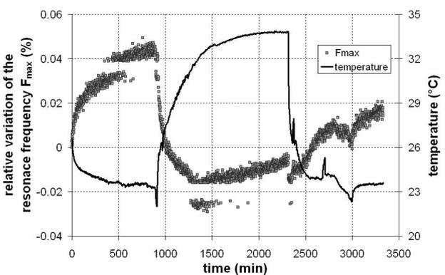
Fig. 7 Temperature dependence of the resonance frequency  $F_{\max}$  for the 0,6mm thin PZ27 piezoelectric cell
