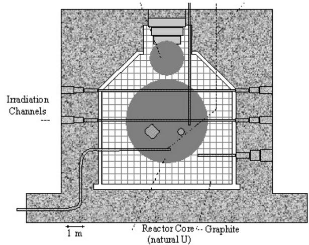
Fig. 10 Schematic structure of the reactor
