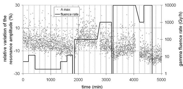
Fig. 3 Effect of gamma radiation for the resonance amplitude of a 2mm thick PZ27 cell
