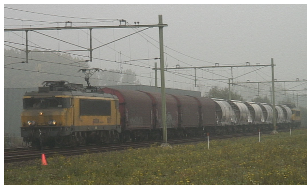
Fig.2 Photo of the test train passing the measurement site. Here, the locomotive is hauling K-block braked Shimms wagons and Tapps wagons, some of which were equipped with wheel dampers.
