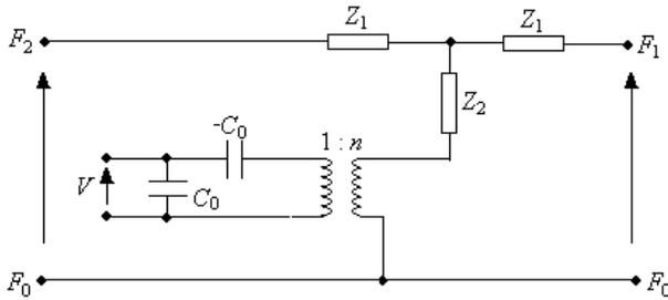
Fig. 1. Mason's circuit model of a piezoelectric ceramic.
