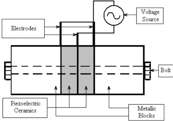
Fig. 4. Schematic representation of the transducer used in the experiments.
