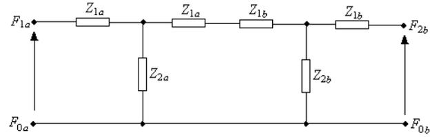
Fig. 5. Network of mechanical load used in the IB model.
