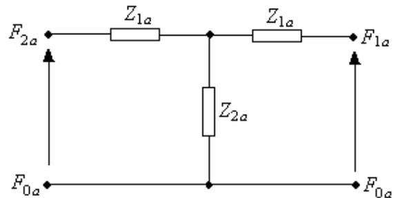
Fig. 3. The circuit model of a passive element.
