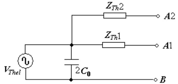
Fig. 2. Complete Thévenin's equivalent circuit.  $B$  is the common terminal.  $A_1$  and  $A_2$  are the points where mechanical parts converted into electric ones are matched.
