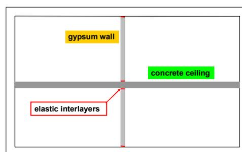
Fig. 6 - two-storeyed combination test facility for the investigation of the vertical flanking transmission
