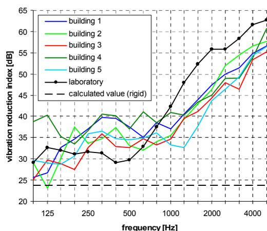
Fig. 9 - vibration reduction index  $K_{ij}$  from gypsum wall to gypsum wall (path Ff) in different buildings and in the laboratory - vertical transmission
