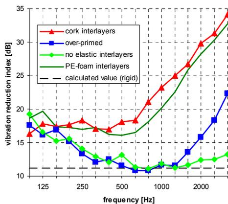
Fig. 7 - vibration reduction index  $K_{ij}$  between gypsum wall and concrete ceiling (transmission path Df respectively Fd) - vertical transmission
