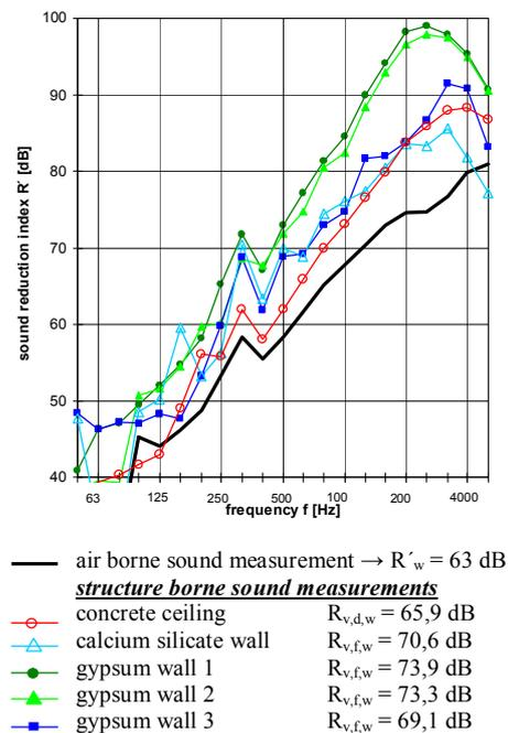
Fig. 8 - sound reduction index of a typical concrete ceiling with the associated flanking reduction indexes
