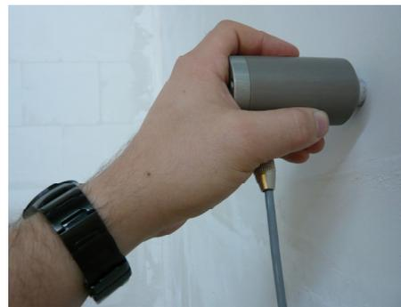
Fig. 2 - small tapping machine for the excitation of the building elements to measure the vibration reduction index
