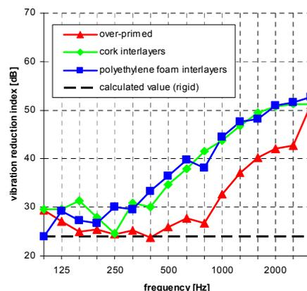
Fig. 5 - vibration reduction index  $K_{ij}$  from gypsum wall to gypsum wall (path Ff) - horizontal transmission
