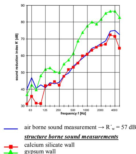
Fig. 4 - sound reduction index of a calcium silicate wall with flanking transmission by a decoupled gypsum wall
