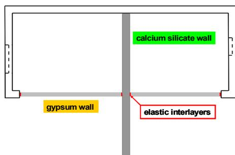
Fig. 3 - test facility for the investigation of the horizontal flanking transmission
