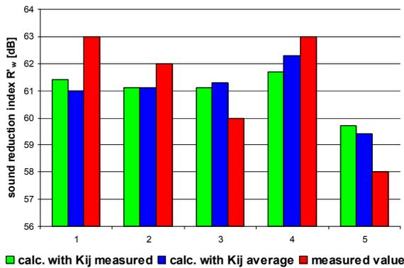
Fig. 10 - sound reduction index - calculated with the simplified model according EN 12354-1 and measured in five different buildings
