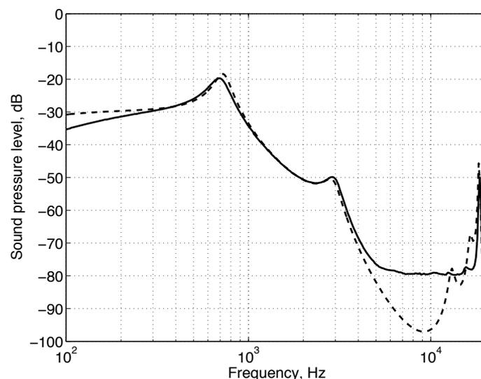
Figure 5: The sound pressure level for the transmission line model with the characteristics of the loudspeaker and the microphone included (- - -), and the measurement result (—) for the test case in figure 3.
