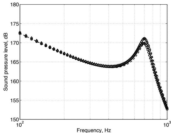
Figure 4: The sound pressure level for the test case in figure 3 with loss included using the transmission line model (- - -), ACTRAN ( $\diamond$ ) and COMSOL ( $\circ$ ).
