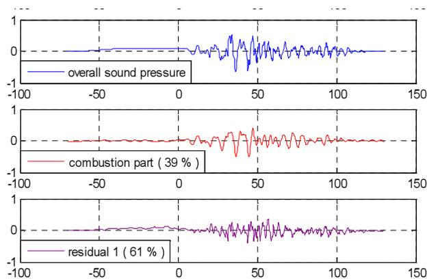
Fig. 3.a. Separation of the combustion noise:
