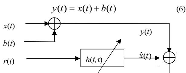
Fig.1 Principle of the cyclic Wiener filtering.
