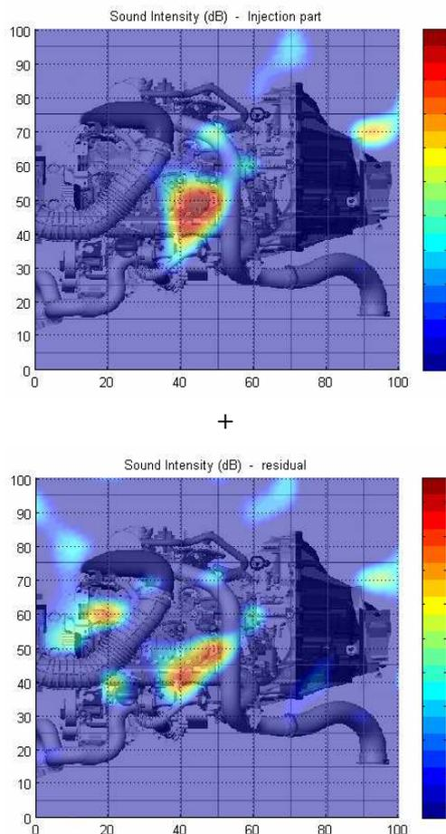
Fig. 4 Separation results for an over face engine: a) global sound intensity, b) combustion part, c) injection part, d) residual.
