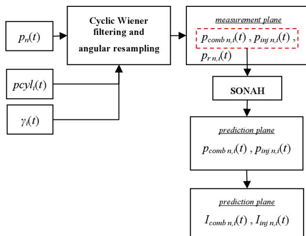
Fig. 2 Process for the calculation of the sound radiation maps.
